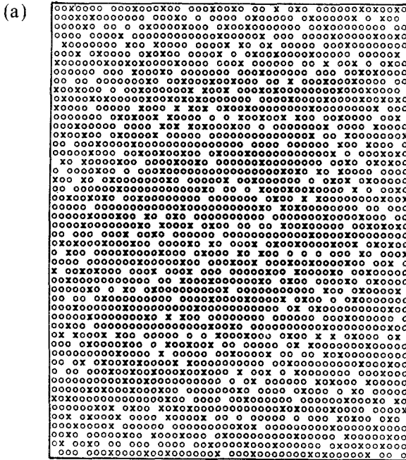
Fig. 2. Typical snapshot configurations of the reactants on the surface characteristic of the model M1. Sample size L = 50 ; (○) A(a), (■) B(a), and (×) AB(a), empty sites are left in white. (a) Saturated surface with A(a) ( \vartheta_A \cong 0.730 ) and AB(a) ( \vartheta_{AB} \cong 0.154 ) after t \cong 10^3 for p_{B_2} = 0.4525 , i.e., just at p_{1B_2} . (b) Configuration obtained during the stationary regime for t = 3 \times 10^3 and slightly above p_{1B_2} , i.e., for p_{B_2} = 0.48 , \vartheta_A \cong 0.308 , \vartheta_B \cong 0.063 , and \vartheta_{AB} \cong 0.113 ; (c) typical configuration obtained when R is maximum for p_{B_2} = 0.51 ( t = 3 \times 10^3 ), \vartheta_A \cong 0.110 , \vartheta_B \cong 0.236 , and \vartheta_{AB} \cong 0.056 ; and (d) configuration obtained during the stationary regime ( t = 3 \times 10^3 ), above the maximum of R and closer to the poisoning transition with B(a) species. p_{B_2} = 0.54 , \vartheta_A \cong 0.042 , \vartheta_B \cong 0.364 , and \vartheta_{AB} \cong 0.03 .
